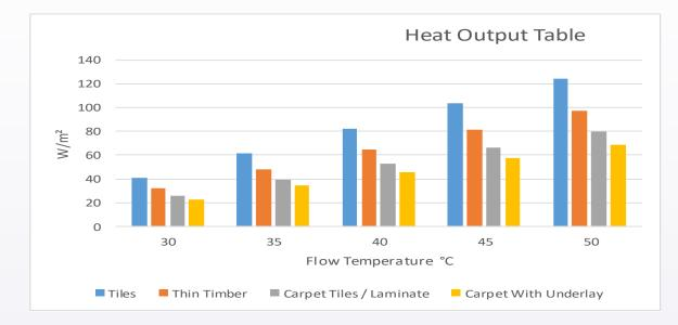
Heat outputs are shown for pipes laid at 200mm centers, with an air temperature of 20°C, more concentrated pipe would increase these figures and less concentrated pipe would have the effect of lowering them.
