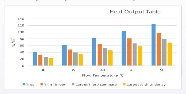
Heat outputs are shown for pipes laid at 200mm centers, with an air temperature of 20°C, more concentrated pipe would increase these figures and less concentrated pipe would have the effect of lowering them.
