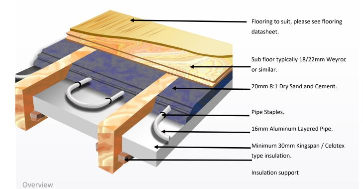
A traditional underfloor heating floor construction used in suspended floors in domestic properties.
