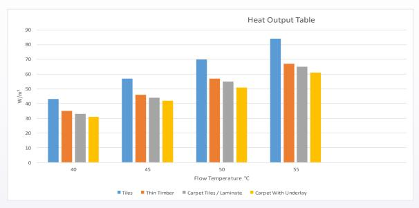
closer together allows for greater outputs for a given flow temperature, or a reduction in flow temperature for a given output.
